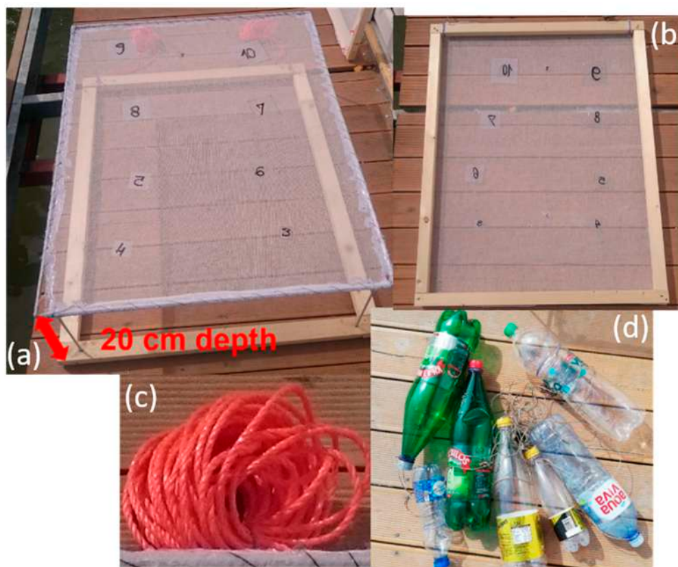
Figure 2. Targets used in the study area located in Lake Balkana (a) frame with metal construction for the underwater survey, (b) frame for the on the water surface survey, (c) nylon rope, (d) plastic bottles.
